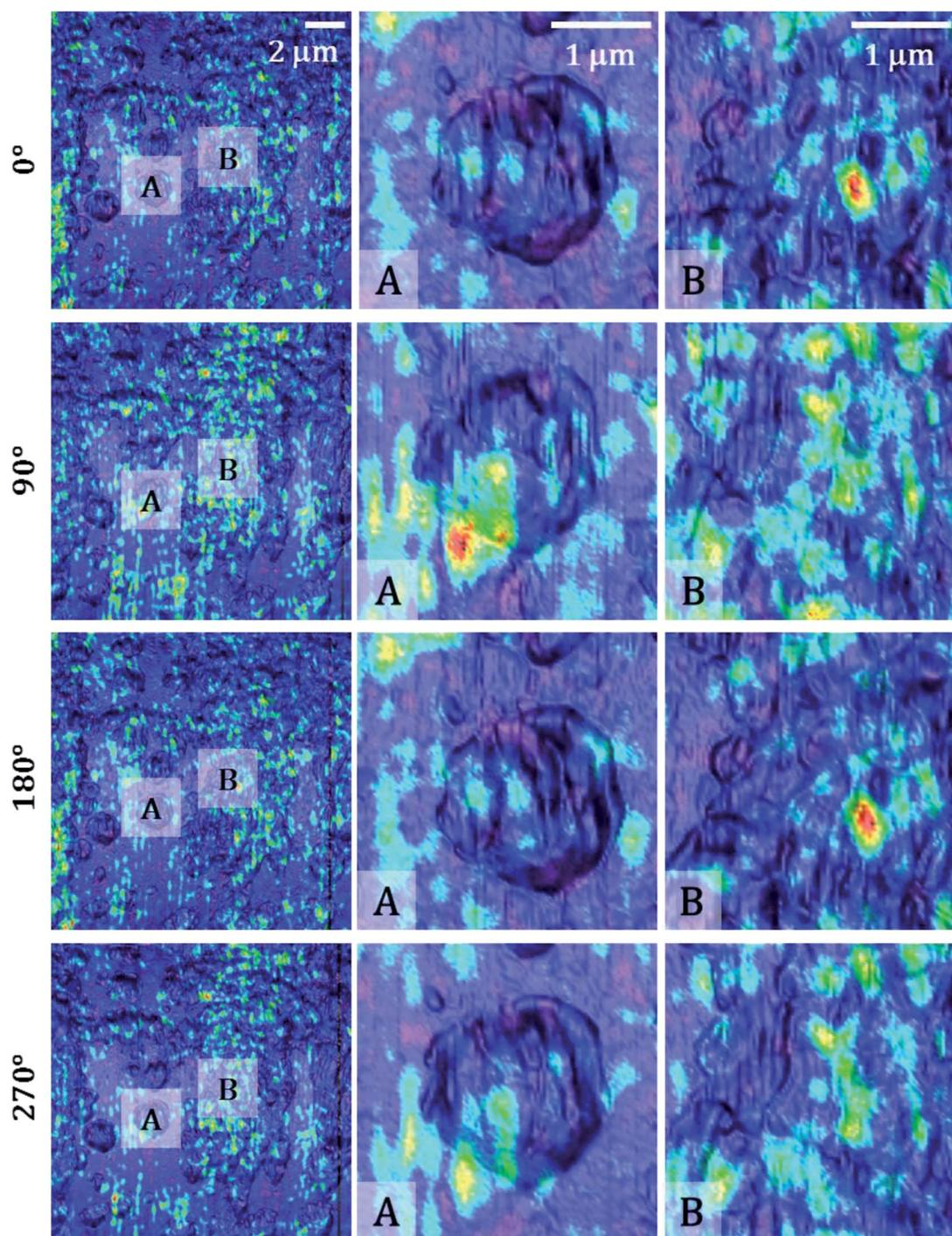
Fig. 5 Polarization dependence of the NSOM signal on the TFBG with randomly deposited nanocubes. Optical  $15 \times 15 \mu\text{m}^2$  images (left column) overlay the topography. Two  $3 \times 3 \mu\text{m}^2$  areas (A and B) were selected to demonstrate a 180 degrees periodicity in the position and intensity of characteristic features. Detailed NSOM images for 12 different polarizations are presented in ESI.†
