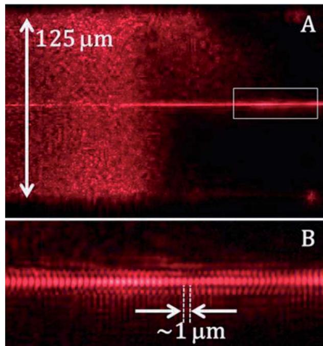
Fig. 2 Far field light microscopy image of light diffracted by a tilted fiber Bragg grating at a wavelength of 647 nm. (A) Light distribution on the TFBG with the left half of the grating covered with silver nanocubes. (B) A zoom of the area indicated in panel A showing the period of  $\sim 1$  micrometer in the diffracted light measured in the far field.
