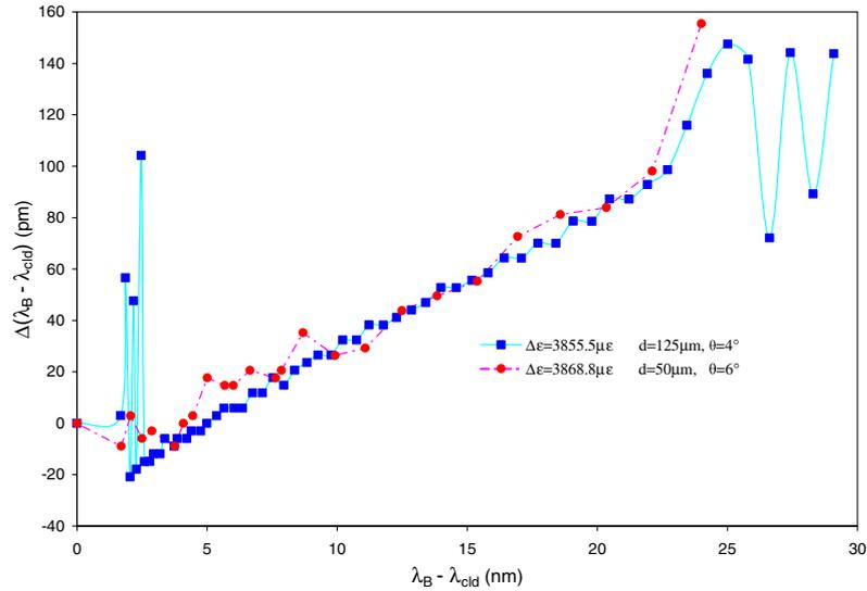
**Figure 4.** Differential wavelength shift of individual resonances for thin and regular fibres near  $3860 \mu\epsilon$ .
