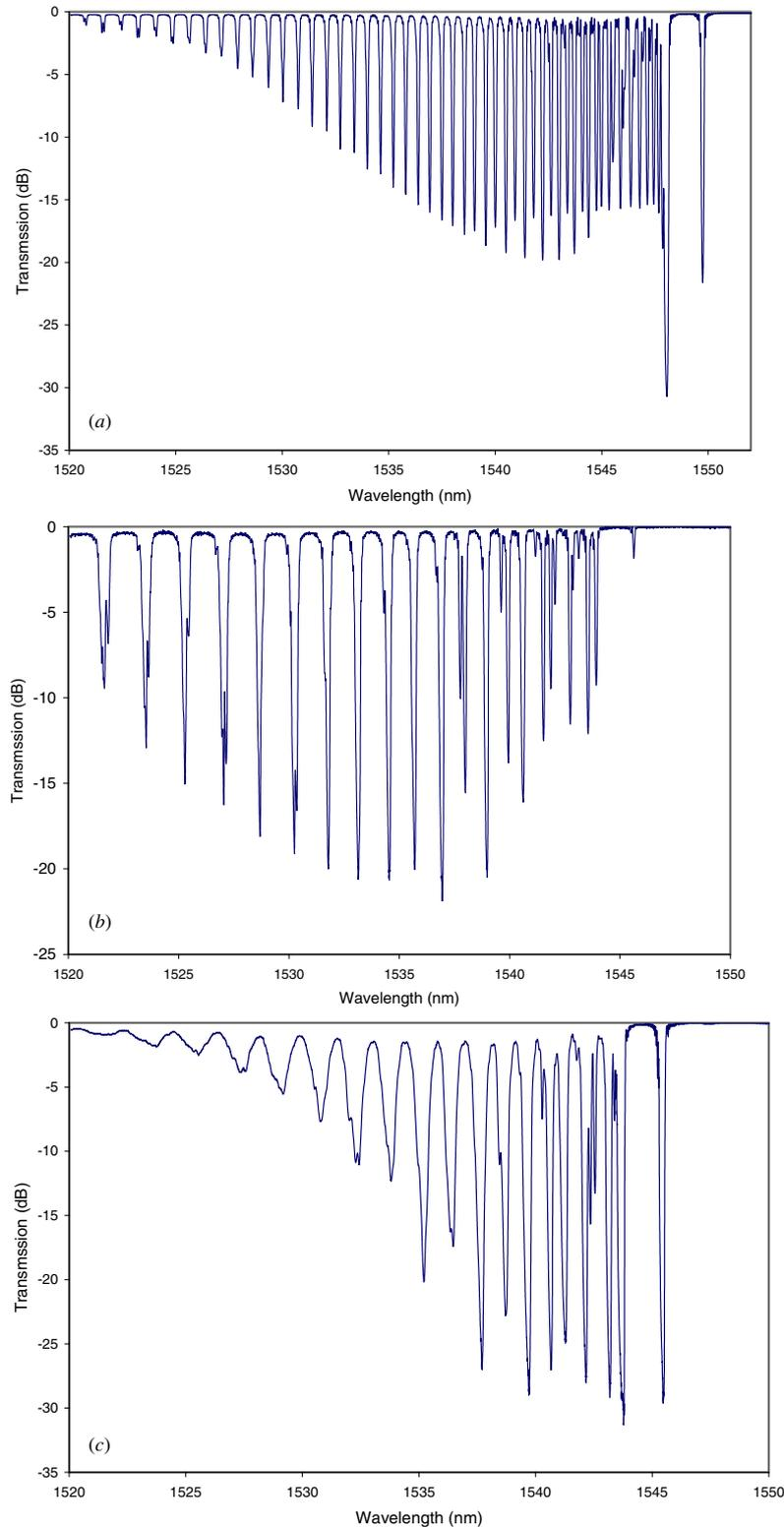
**Figure 1.** The transmission spectra of weakly TFBG: (a) SMF-28 fibre  $d = 125 \mu\text{m}$  and  $\theta = 4^\circ$ ; (b) Corning experimental thin cladding layer fibre  $d = 50 \mu\text{m}$  and  $\theta = 6^\circ$ ; (c) thin cladding layer by HF etching from SMF-28 fibre  $d = 50 \mu\text{m}$  and  $\theta = 4^\circ$ .
