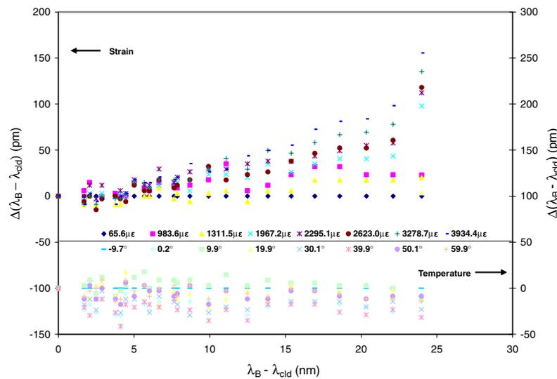
**Figure 3.** The relative wavelength shift of cladding mode resonances to the Bragg resonance of TFBG with thin cladding layer  $d = 50 \mu\text{m}$  and  $\theta = 6^\circ$  due to longitudinal strain and temperature perturbations.
