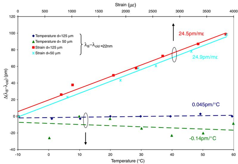
**Figure 5.** Comparison of differential wavelength shifts of cladding mode resonances for a  $4^\circ$  tilted FBG in SMF-28 fibre and a  $6^\circ$  tilted FBG in Corning experimental  $50 \mu\text{m}$  diameter thin cladding fibre  $\sim 22 \text{ nm}$  away from their Bragg resonances due to strain and temperature perturbations.
