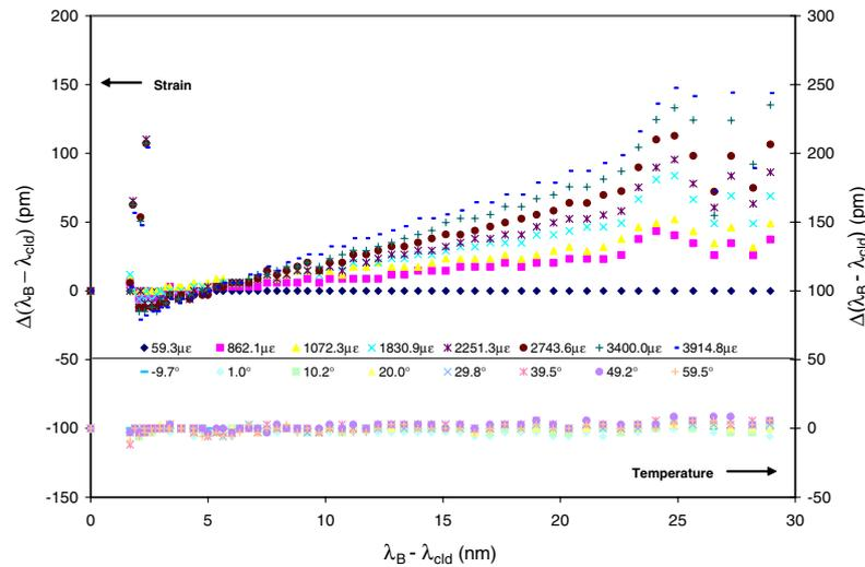
**Figure 2.** The relative wavelength shift of cladding mode resonances to the Bragg resonance of TFBG with standard SMF-28 fibre  $d = 125 \mu\text{m}$  and  $\theta = 4^\circ$  due to longitudinal strain and temperature perturbations.
