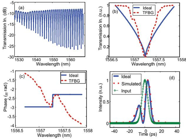
Fig. 1. (a) Transmission spectrum of a TFBG with a tilt angle of  $10^\circ$ . (b) Magnitude response. (c) Phase response of one channel of the TFBG. The solid line shows the magnitude and phase response of an ideal differentiator. (d) Simulated output pulse from the TFBG. The dotted line shows the output pulse from an ideal differentiator. The fractional order is 0.675. In.: Intensity.
