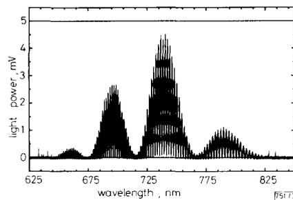
Fig. 3 Output power of coupled arm for two cascaded Mach-Zehnders with central spacing 26.5 mm and 105 mm between coupler centres
