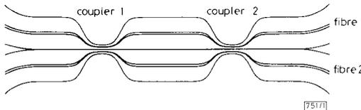
**Fig. 1** Unbalanced dissimilar-fibre Mach-Zehnder
