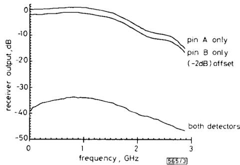
**Fig. 3** Frequency response of receiver and noise cancellation
