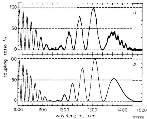
Fig. 2 (a) measured and (b) calculated coupling ratio against wavelength for Mach-Zehnder made from identical 1-cycle couplers with 53 mm spacing between coupler centres
