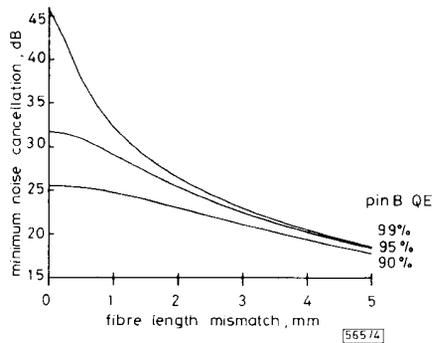
**Fig. 4** Minimum noise cancellation for 565 Mbit/s dual-detector receiver
