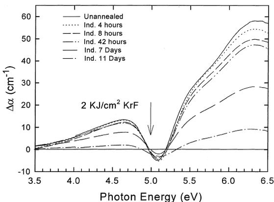
Fig. 3. Induced absorption coefficient spectra following 2 KJ/cm<sup>2</sup> of KrF irradiated unannealed and annealed 3GeO<sub>2</sub>:97SiO<sub>2</sub> glasses for different periods of time. Each spectrum results from the difference of that obtained after irradiation to that before irradiation.
