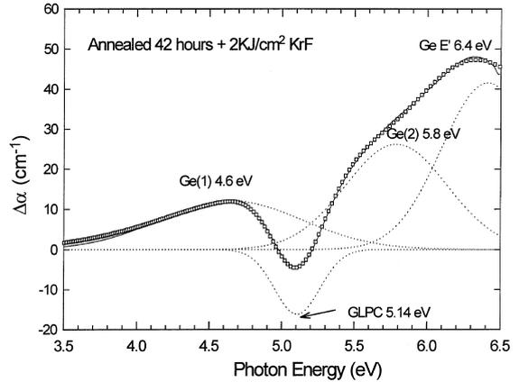
Fig. 4. Deconvolution of the induced absorption spectrum measured after 42 h of annealing and irradiation with 2 kJ/cm<sup>2</sup> KrF laser light. Open squares denote the experimental data, solid lines are the fitted result and the dashed lines denote the separate Gaussian components.
