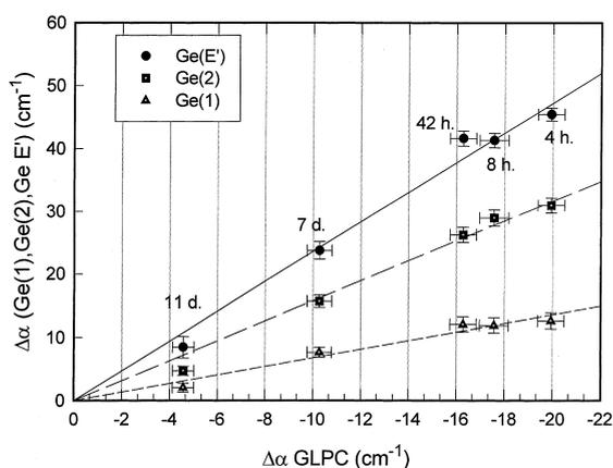
Fig. 6. Correlation between the bleaching of the GLPC (5.14 eV) and the growth of the Ge(1)(4.6 eV), Ge(2)(5.8 eV) and Ge E' (6.4 eV) absorption bands at the same dose of laser irradiation of samples annealed for different periods of time.
