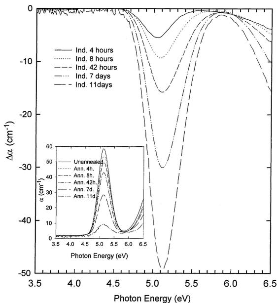
Fig. 1. Induced absorption spectra of  $3\text{GeO}_2:97\text{SiO}_2$  glasses after annealing at  $1000^\circ\text{C}$  under a continuous flow of oxygen for 4, 8, 42 h, 7 and 11 days. The absorption spectrum of the unannealed sample is subtracted from those of the annealed samples which are shown in the inset.
